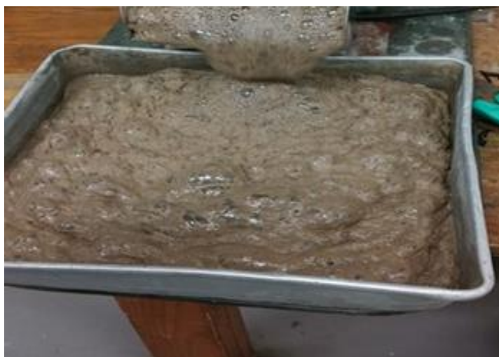
Figure 4.17. A picture of froth products collected at longer residence time (0 to 10 min) when sodium silicate dispersant was used.
