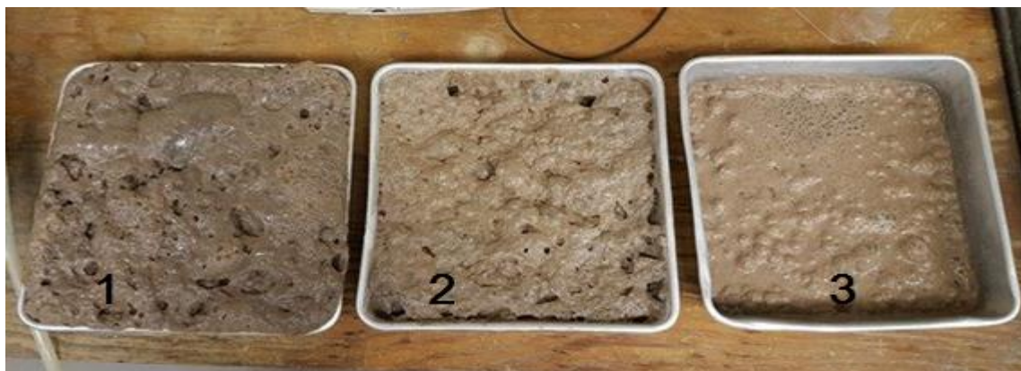
Figure 4.16. A picture of froth products collected at different time ranges when sodium silicate dispersant was used 1) 0 to 2 min, 2) 2 to 4 min, and 3) 4 to 6 min.
